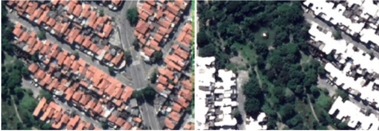
Figure 2 | Example of image sample example on the left, used in roof area estimates, and the result of segmentation on the right.
