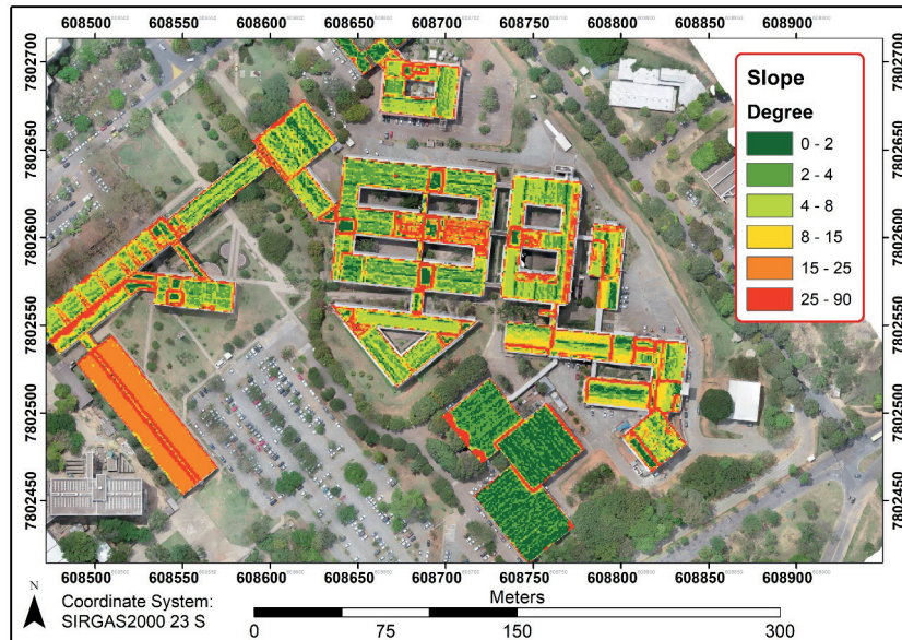
Figure 5 | Slope of the roofs of EE-IGC-UFGM.
