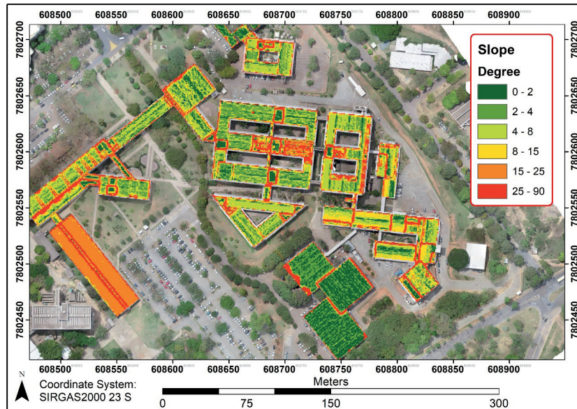
Figure 5 | Slope of the roofs of EE-IGC-UFGM.
