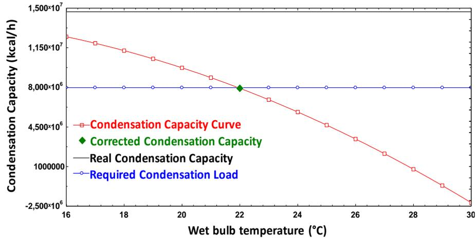
Figure 4. Thermal capacity with all condenser running.
