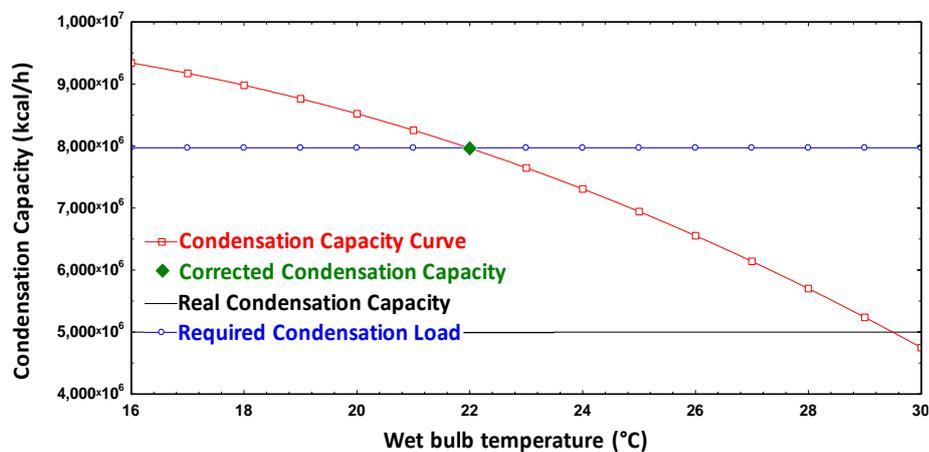
Figure 3. Real Thermal capacity verified
