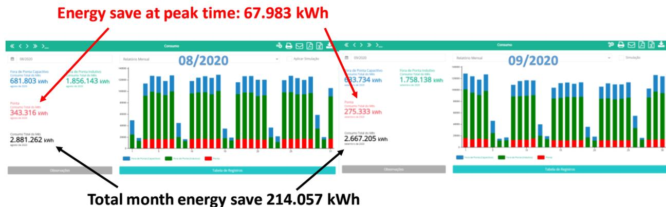
Figure 8. Comparison monthly energy consumption between August and September of 2020
