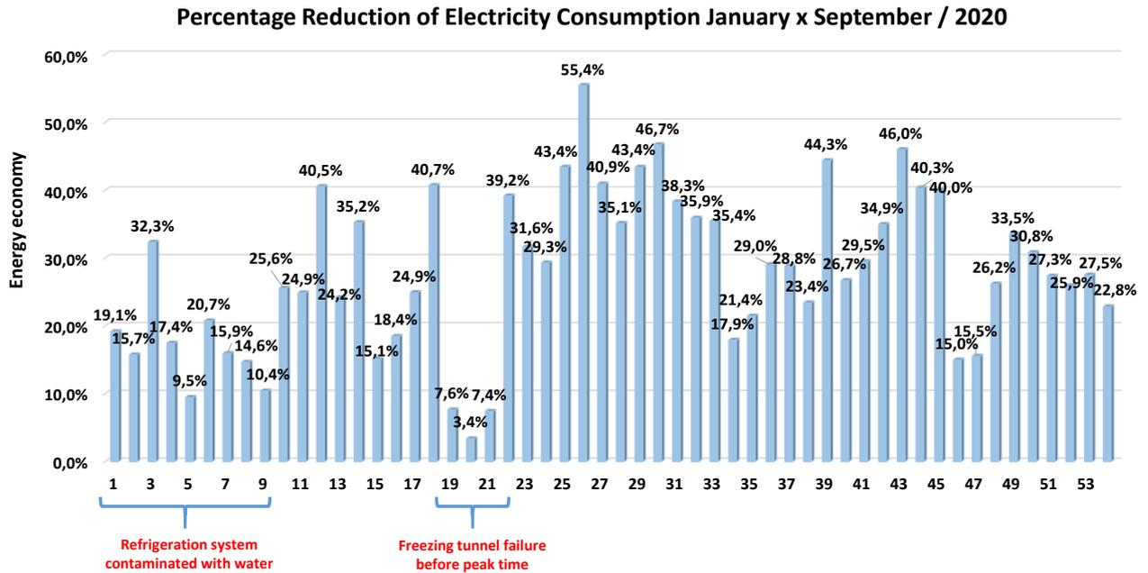
Figure 5. Real electrical energy reduction in relationship January/2020.
