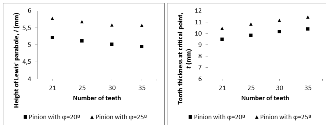
Figure 11 – Height of Lewis' parabole ( l ) and tooth thickness at critical point ( t ).
