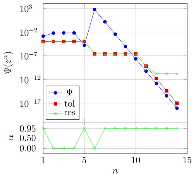
**Figure 4: Newton method convergence: Residual for each iteration( $\Psi$ ), solver tolerance (tol), relative solver residual (res), and  $\alpha$  obtained on line search.**
