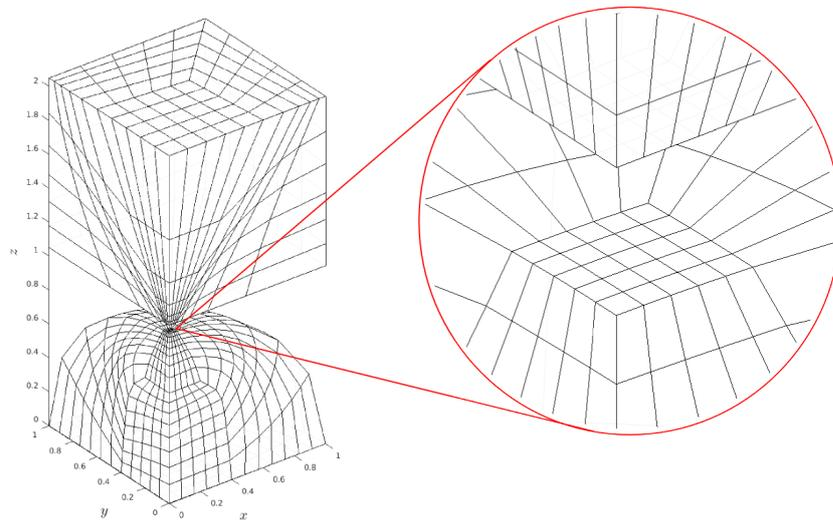
Figure 3: Mesh used on the Hertzian contact example
