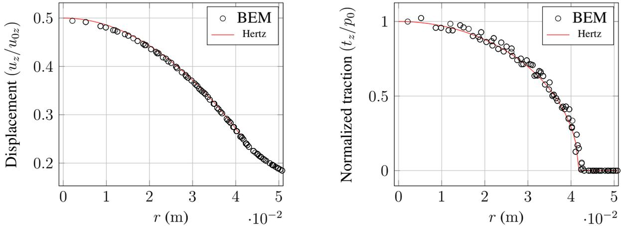
(a) Displacements along contact region relative to displacement applied.
