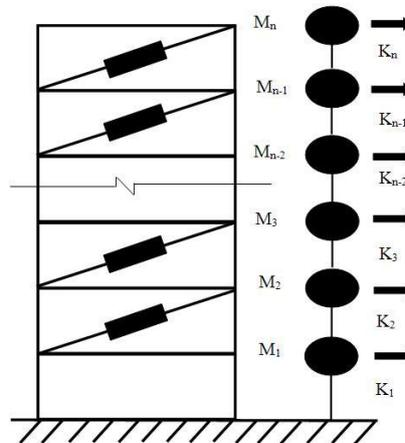
Figure 3. Schematic model of a shear building represented as lumped mass system.
