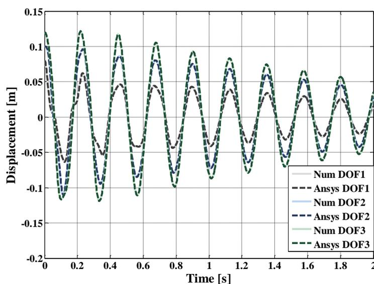
Figure 2. Comparison of response between ANSYS and the proposed numerical method
