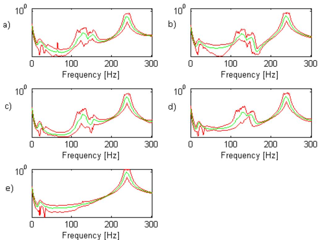
**Figure 6. Mean value and upper and lower 95% percentile from the measured FRFs on positions (a) 1, (b) 2, (c) 3, (d) 4 and (e) 5.**
