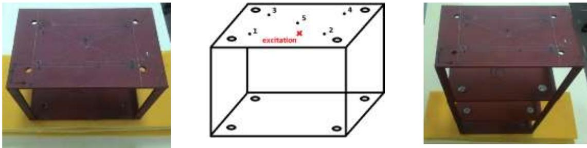
**Figure 1.** Picture of single frame test setup (left), schematic frame draft (middle) and picture of one assembly (right).
