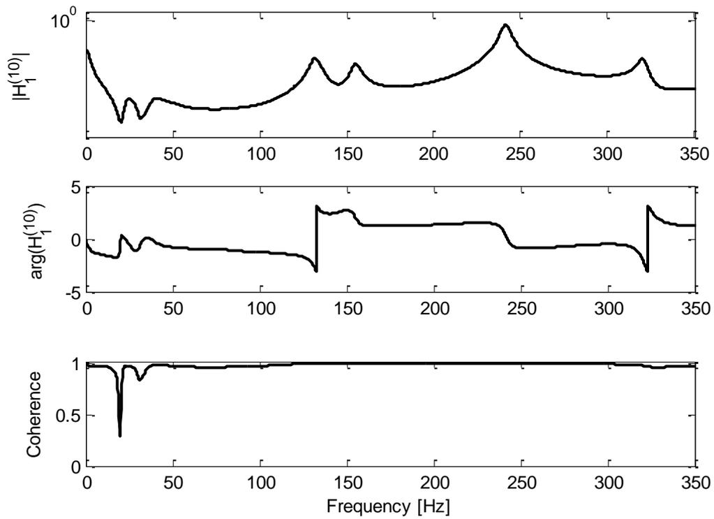
Figure 3. FRF modulus, phase and coherence of component #10 measured at point 1
