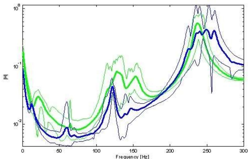
**Figure 9.** Mean FRFs (thick) and respective percentiles (thin) of component (green) and ensemble (blue)
