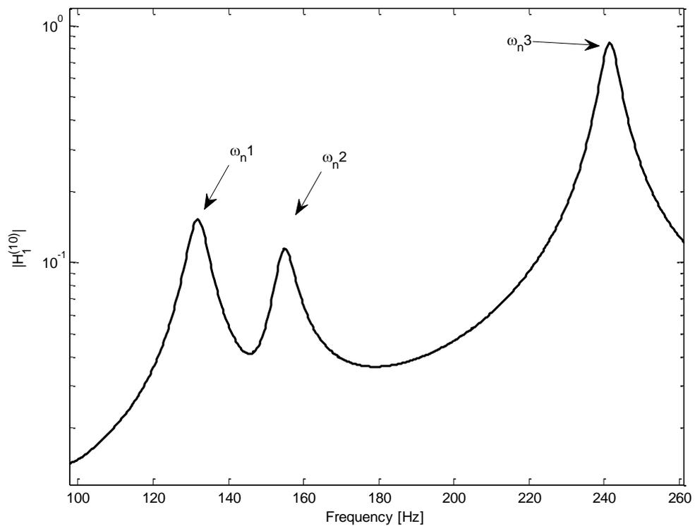
Figure 4. FRF of component #10 with analyzed frequencies pointed
