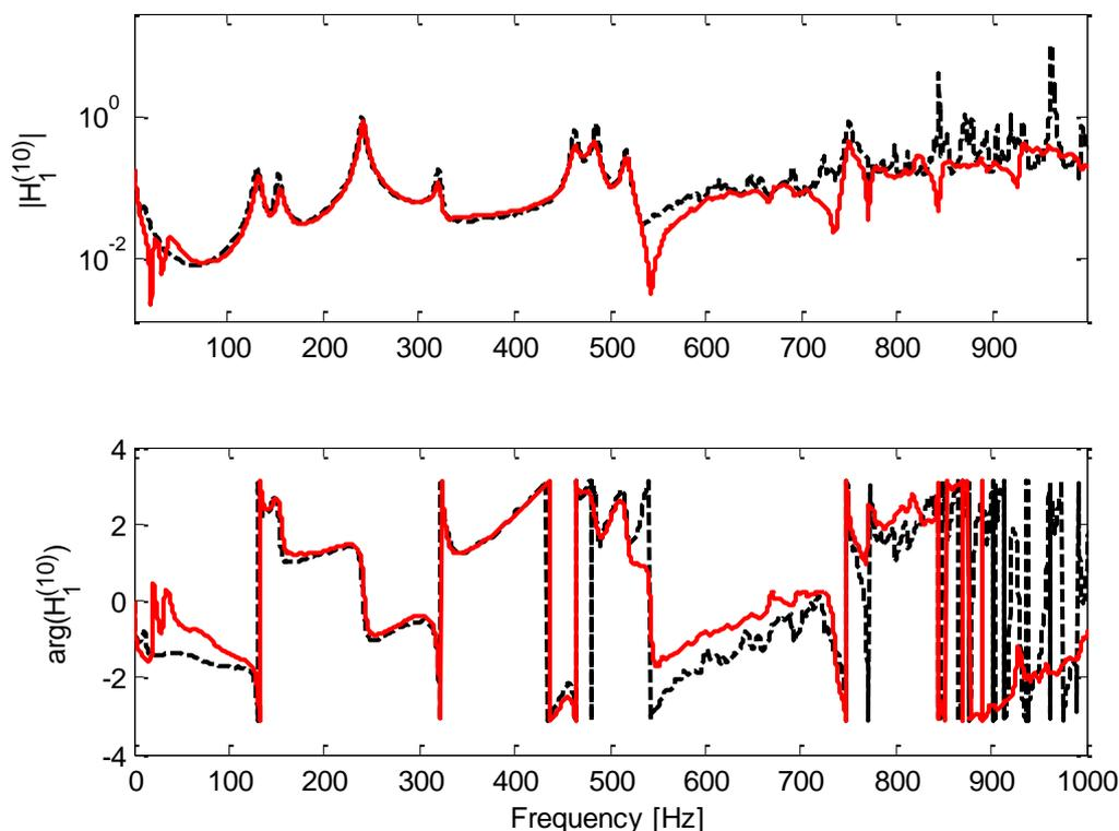
**Figure 2. Typical amplitude and phase of the FRFs from a frame tested on foam (red) and hang by strings (black).**
