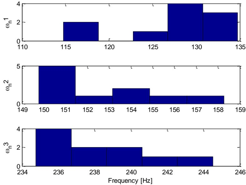
Figure 7. Experimentally obtained histogram of the natural frequencies from the ensemble of components.
