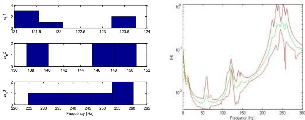
**Figure 8.** Experimentally obtained histogram from the natural frequencies (left) and 95% upper and lower percentile of the frequency response (right) from the assemblies.
