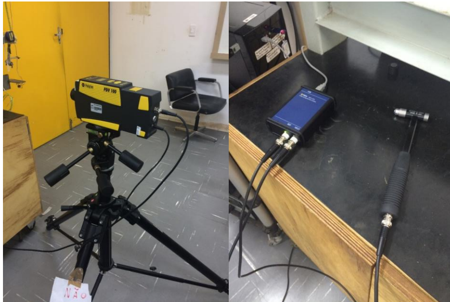
Figure 1. LDV Polytec PVD 100 (left) and PCB 086C01 modal hammer and acquisition board used (right).
