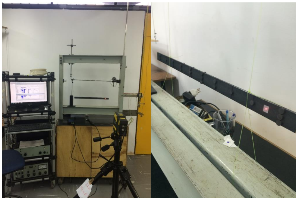
Figure 2. Experimental setup including modal hammer, LDV, acquisition system, and the hung beam(left) and a details of a sample configuration of the attached magnets and measuring point (right).
