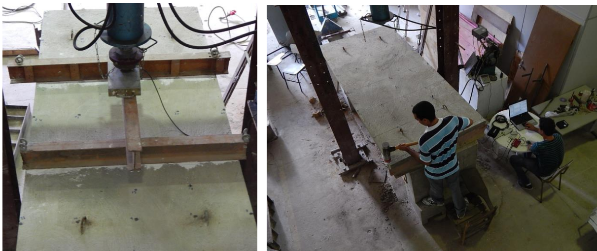
(a) Load distribution by a hydraulic jack.
