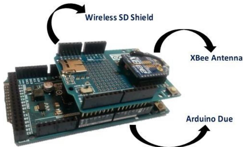
Figure 2. Arduino Due + Wireless SD Shield + Antenna
