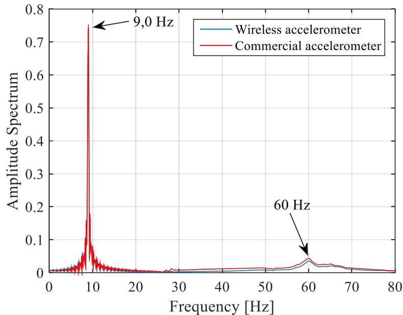
Figure 7. FFTs obtained by the low-cost wireless accelerometer and the commercial accelerometer
