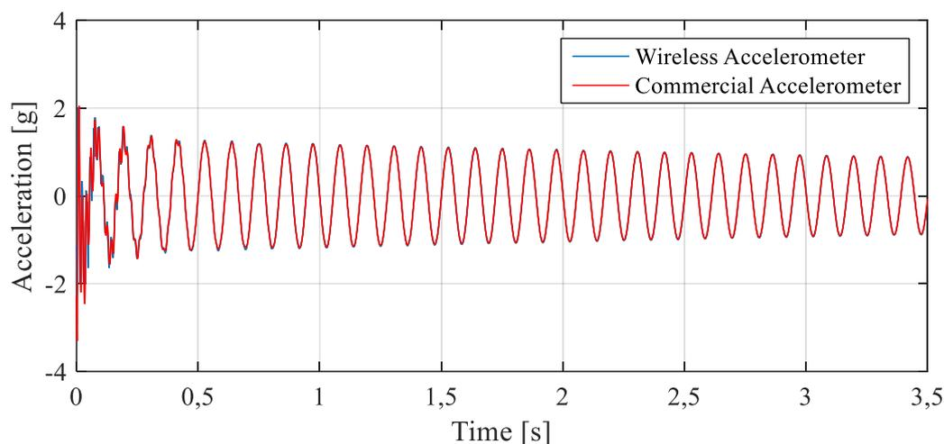
Figure 5. Signals acquired by both accelerometers (from 0 to 3,5s).
