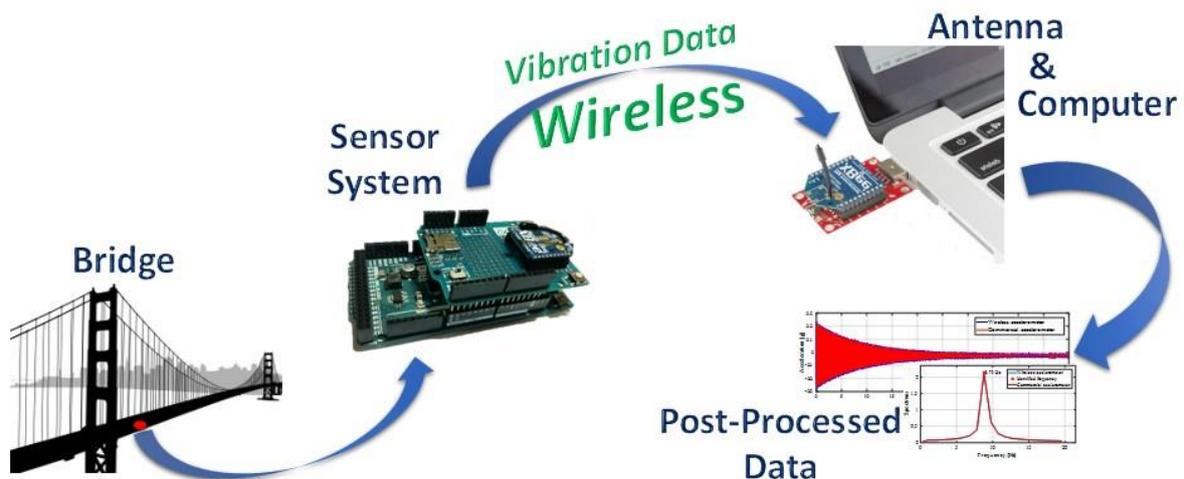
Figure 1. Wireless system schematic
