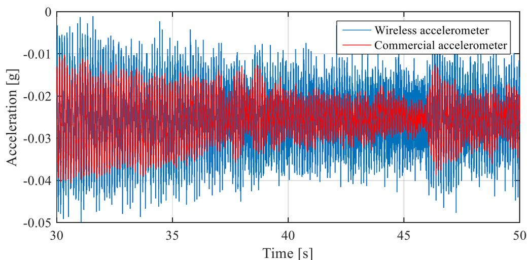
Figure 6. Signals acquired by both accelerometers (from 30 to 50s).
