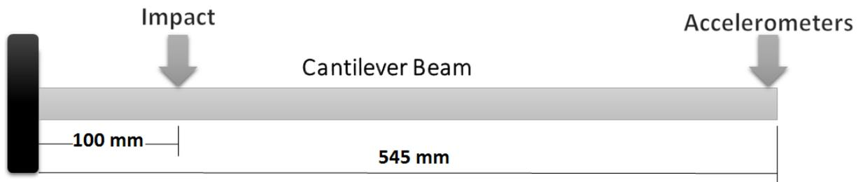
Figure 4. Cantilever beam.
