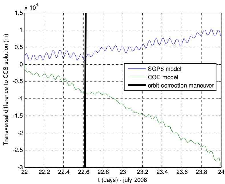
**Figure 6. SGP8 and COE models propagation difference to SCC orbit determination solution based on transversal data in radial direction**
