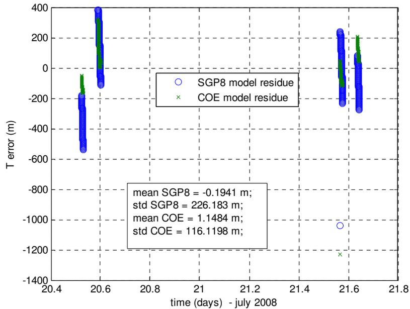
**Figure 3. Position residue in transversal direction. Residue statistics (mean and standard deviation) are also shown for the two models**
