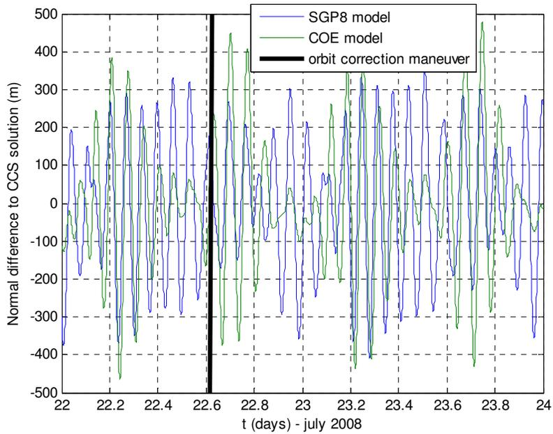
**Figure 5. SGP8 and COE models propagation difference to SCC orbit determination solution based on normal data in normal direction**
