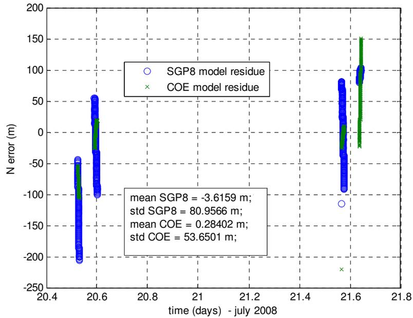
**Figure 2. Position residue in normal direction. Residue statistics (mean and standard deviation) are also shown for the two models**
