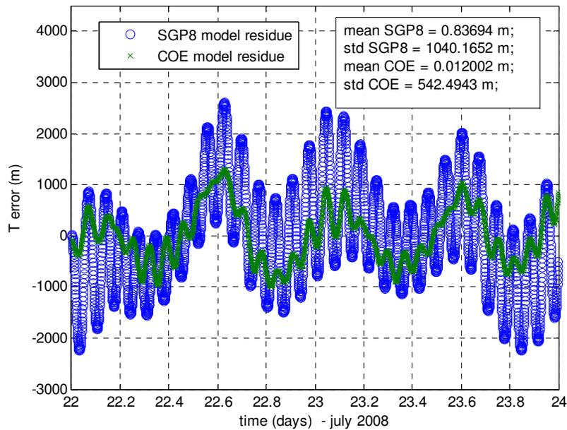
**Figure 9. Position residue in transversal direction - identification with radar data. Residue statistics (mean and standard deviation) are also shown for the two models**
