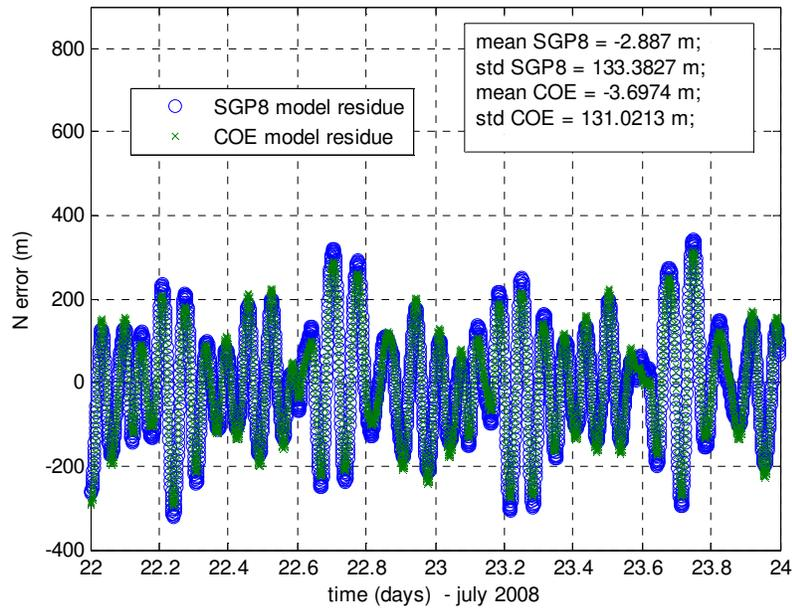
**Figure 8. Position residue in normal direction - identification with radar data. Residue statistics (mean and standard deviation) are also shown for the two models**
