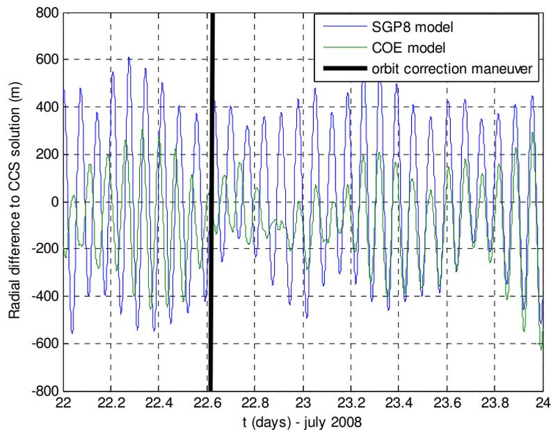
**Figure 4. SGP8 and COE models propagation difference to SCC orbit determination solution based on radar data in radial direction**
