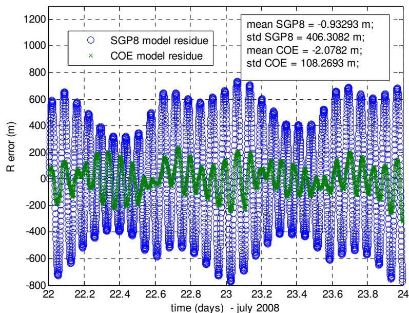
**Figure 7. Position residue in radial direction - identification with radar data. Residue statistics (mean and standard deviation) are also shown for the two models**
