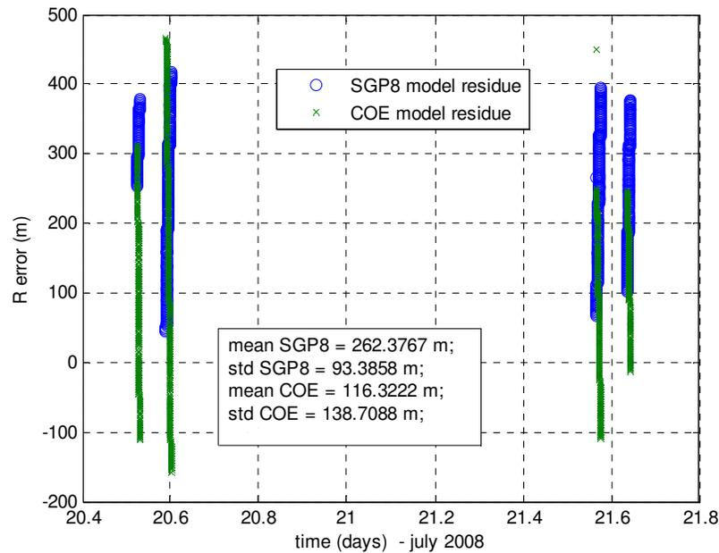
**Figure 1. Position residue in radial direction. Residue statistics (mean and standard deviation) are also shown for the two models**
