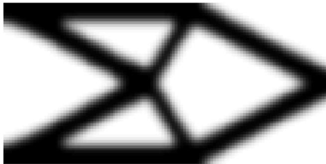
**Figure 3: Optimum design for the cantilever beam ( $120 \times 60$  mesh).**
