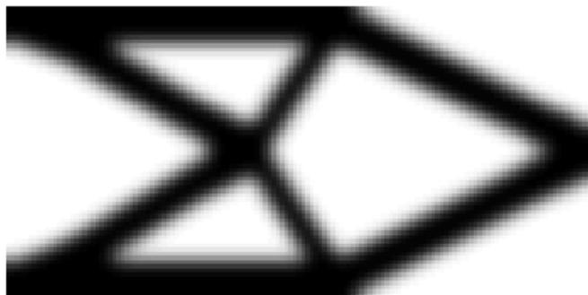
**Figure 4: Optimum design for the cantilever beam ( $140 \times 70$  mesh).**
