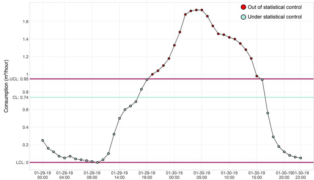
**Figure 6:** EWMA control chart – Joinville branch hourly consumption from January 29 to 30, 2019.
