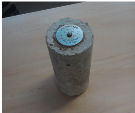
Figure 2 . Inlaid plate on a concrete pillar.
