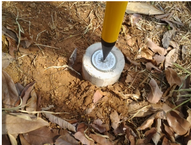
Figure 4. Metal plate carved in concrete block.
