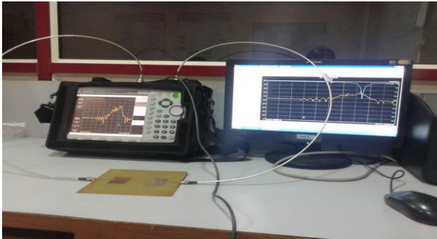
Figure 11 – Experimental set up of V.N.A.
